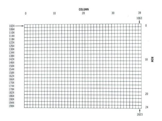
The 64's screen memory normally begins at memory location 1024 and ends at location 2023. Location 1024 is the upper left corner of the screen. Location 1025 is the position of the next character to the right, and so on. Location 1063 is the right-most position of the first row. Following the last character in a row, the next location is the left-most character on the next row down.
