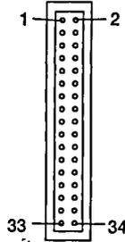
Figure 3-132 shows the voltages and signals assigned to the diskette drive connector.
