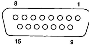
**Figure 4-2. Power/Audio Cable Connector**
