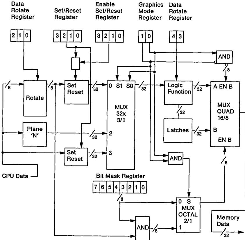
Figure 3-29. Data Flow for VGA Memory Write Operations
