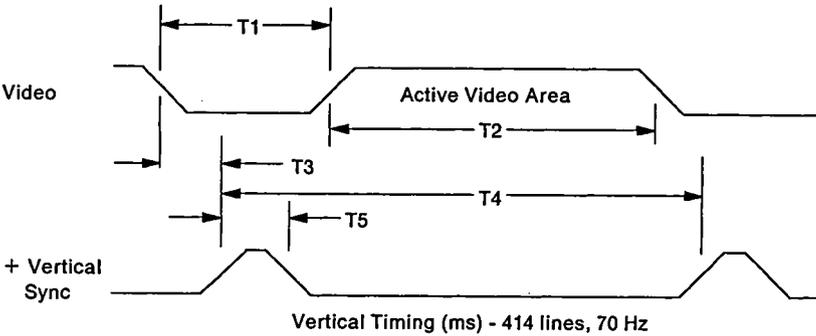
**Figure 3-94. Display Vertical SYNC, 400 Lines
