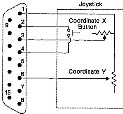
Note: Potentiometer for Coordinates X and Y has a range of 0 to 145 k-ohms. Button is normally open; closed when pressed.
