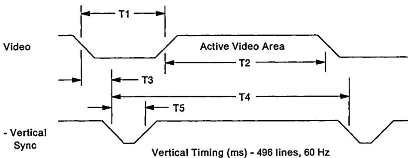
**Figure 3-95. Display Vertical SYNC, 480 Lines
