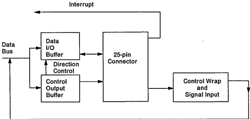
Figure 3-147. Parallel Port Controller Block Diagram
