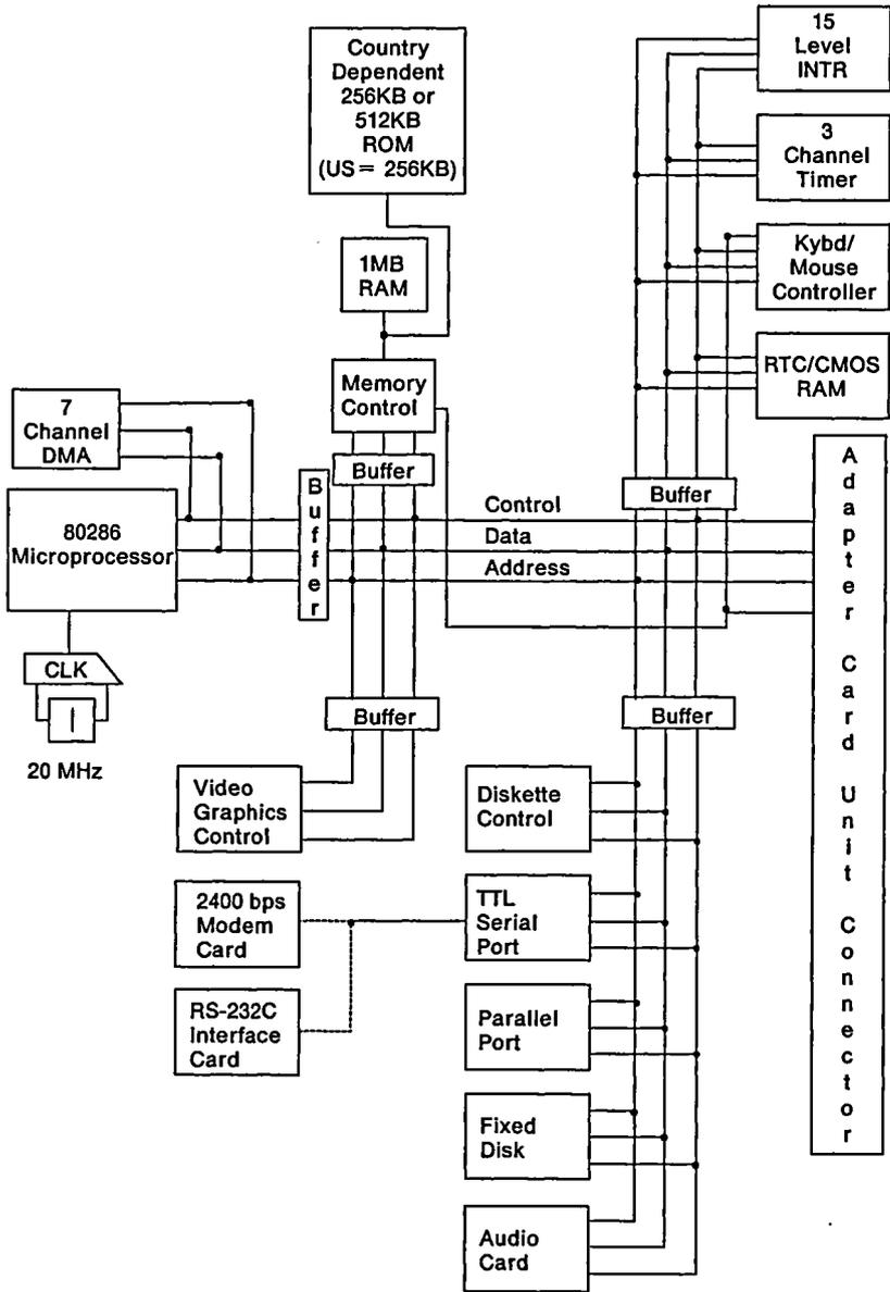
Figure 1-2. System Board Block Diagram
