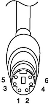
*Figure 6-50. Mouse Connector Pin Assignments*
