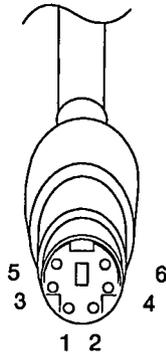
*Figure 5-24. Keyboard Connector Signal and Voltage Assignments*
