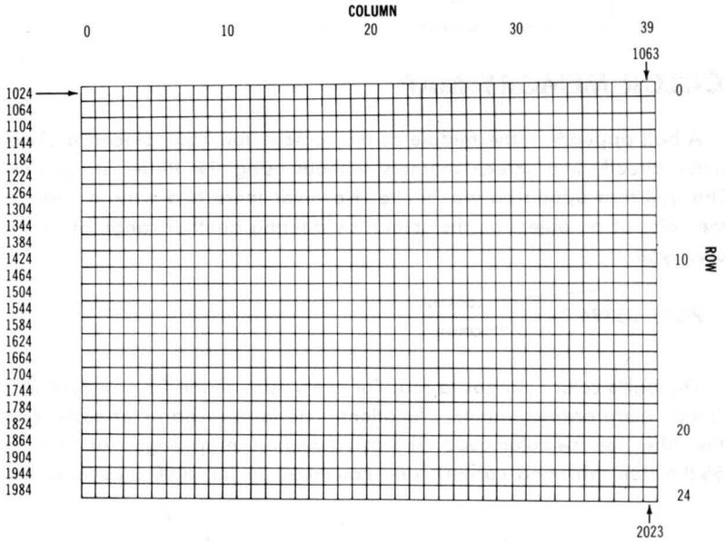
Screen memory in the Commodore 64 normally begins at memory location 1024, and ends at location 2023. Location 1024 is the upper left corner of the screen. Location 1025 is the position of the next character to the right of that, and so on down the row. Location 1063 is the right-most position of the first row. The next location following the last character on a row is the first character on the next row down.
