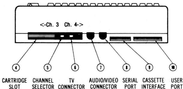
9. **Cassette Interface.** A DATASSETTE recorder can be attached to the computer so you can save information entered for use at a later time.
