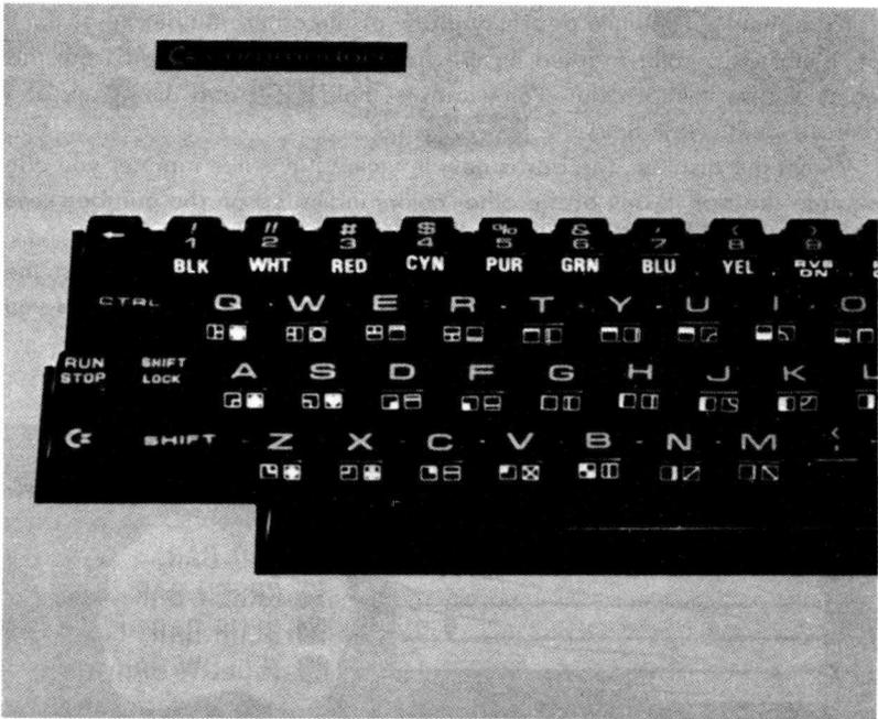
To use a control function, you hold down the **CTRL** key while depressing a second key.
