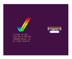
You can then insert either a Workbench disk or any other bootable disk such as a game into the floppy drive on the right-hand side of the Amiga (called DF0: - Disk Floppy Zero).
