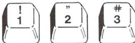
When you are using the graphics on the front of the keys, the SHIFT key displays the graphic character on the **RIGHT** side of the key.
