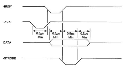
Figure 3-153. Parallel Port Timing Sequence
