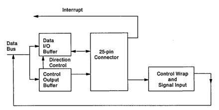
Figure 3-147. Parallel Port Controller Block Diagram
