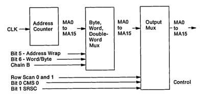
Figure 3-64. CRT Controller Memory Address Mapping
