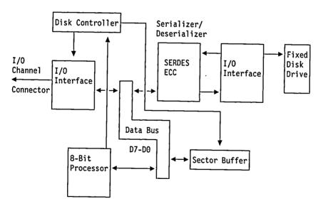
Figure 8-1. Fixed Disk and Controller
