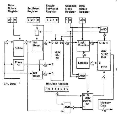
Figure 3-29. Data Flow for VGA Memory Write Operations
