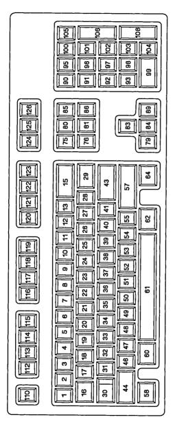
Figure 5-1. Key Numbering for the 101-Key Keyboard
