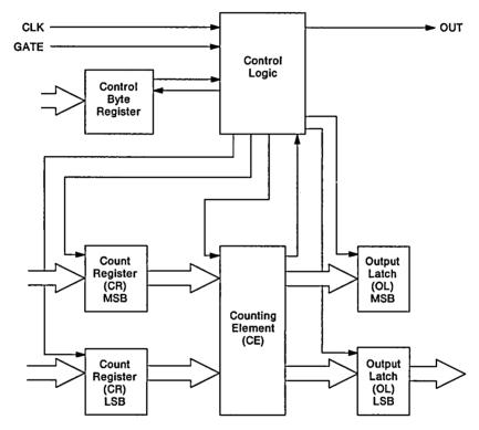
Figure 2-15. System Timer Block Diagram
