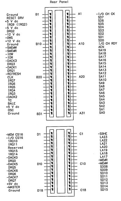
Figure A-10. I/O Channel Connectors.
