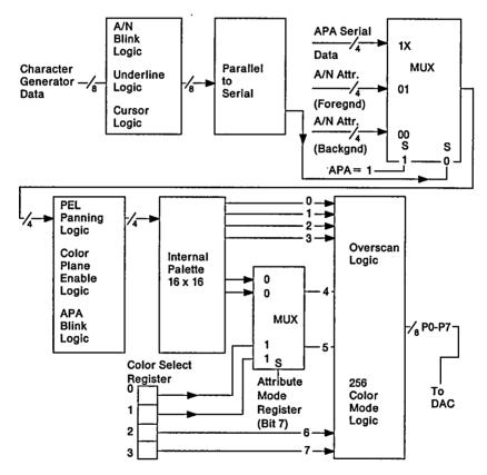
Figure 3-12. Attribute Controller Block Diagram
