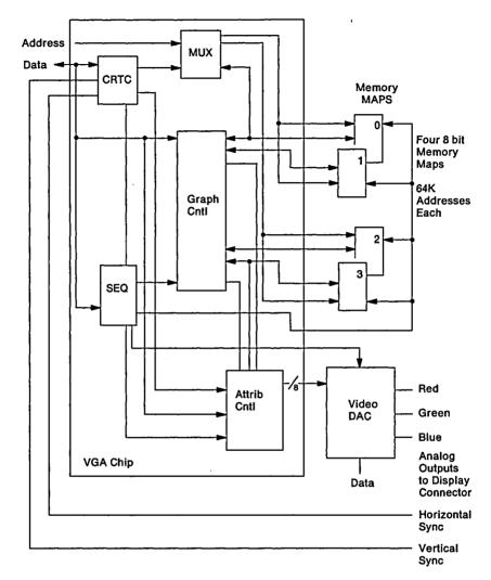
Figure 3-10. Video Subsystem Block Diagram
